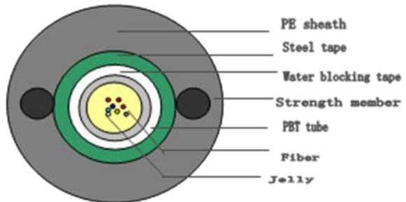
Application: Duct, direct buried, tunnel and non-messenger aerial
